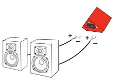
\* Connect your speakers in parallel. Make sure the positive wires and the negative wires are connected together in the same speaker connector.
