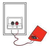
**B.** Connect the cables from the speaker into the speaker connectors of The Vamp\*.
